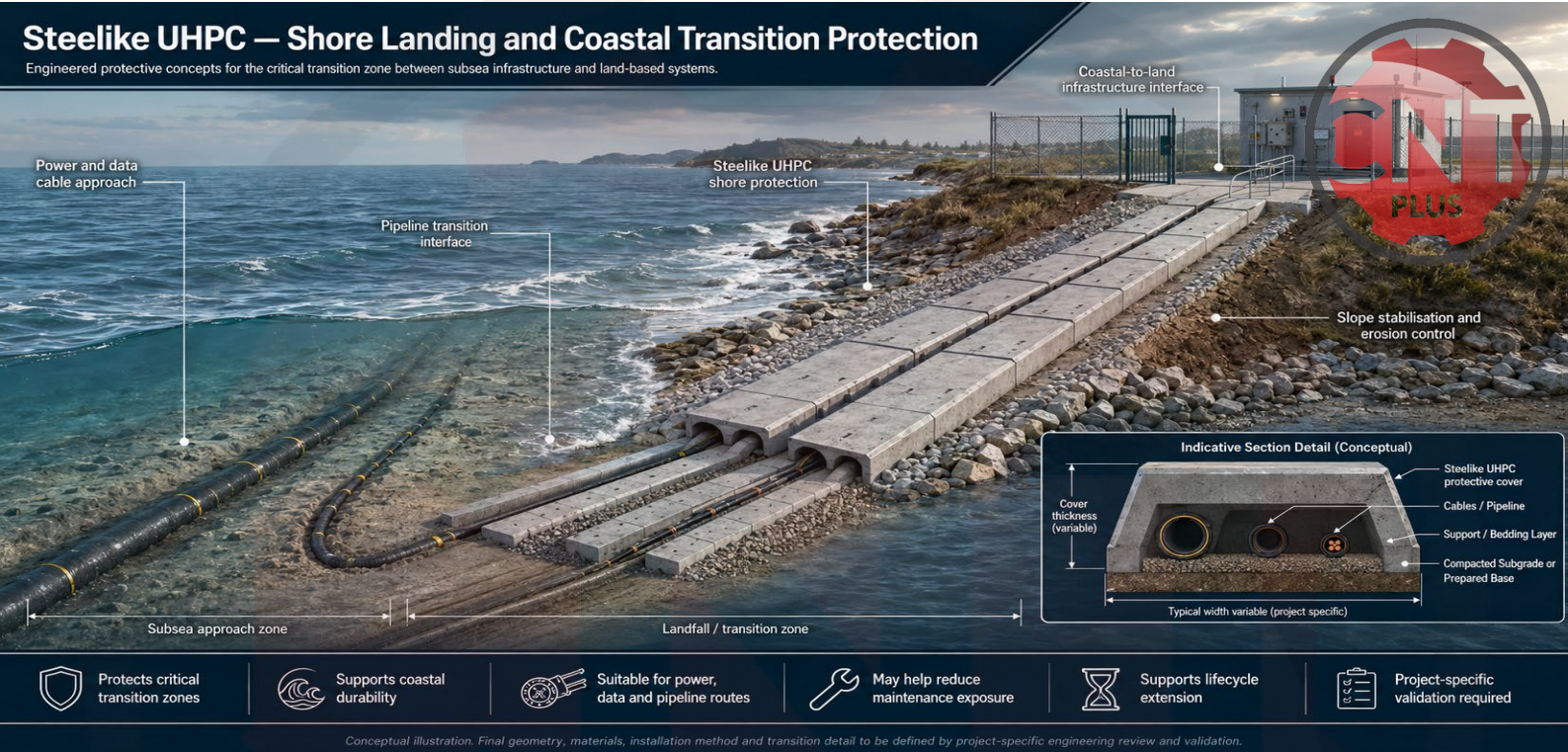
Figure 1. Shore landing and coastal transition protection concept. Conceptual Steelike UHPC protective arrangement for the critical transition zone between subsea pipeline, power cable or data cable corridors and land-based infrastructure. Final geometry, cover thickness, bedding layer, installation method and acceptance criteria require project-specific engineering review and validation.
